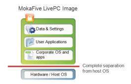
The LivePC image is completely isolated from, and independent of, the underlying host machine. Although the virtual machine "borrows" what it physically needs from the host (CPU, RAM, keyboard, mouse, monitor, etc.), the operating system, applications and data are kept separate. Viruses and malware on the host are not able to infect the virtual machine, and the virtual environment does not leave a trace of data on the device once shut down.
